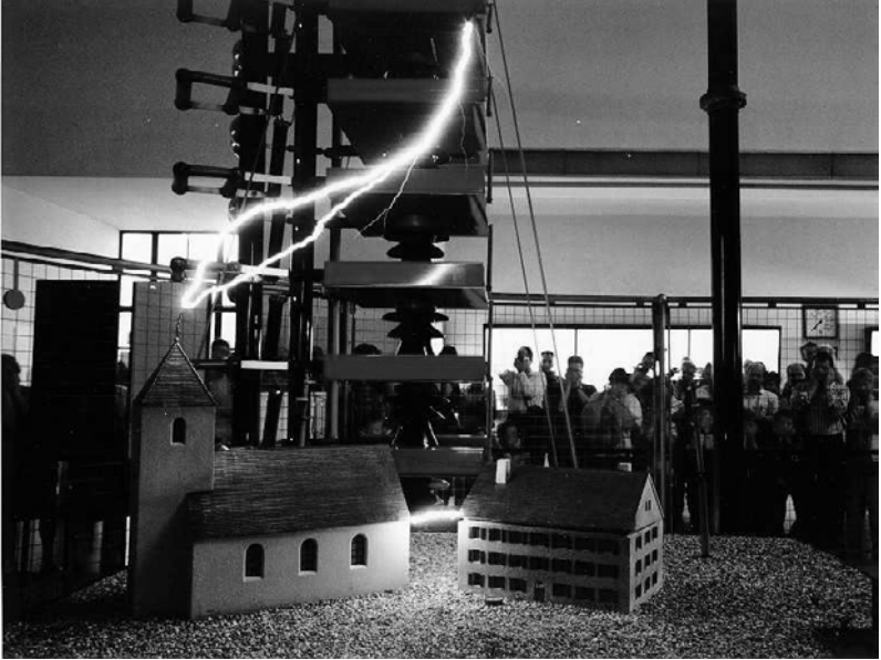
Figure 4-4. Lightning demonstration at the Deutsches Museum in Munich. 11 In this demonstration, a lightning bolt strikes a church that is not well grounded. Because the church is not well grounded, a second stroke occurs between the church and a nearby house.
